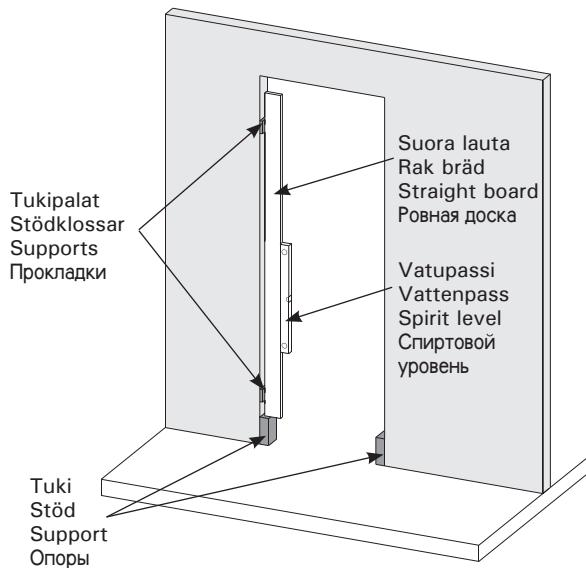
3. Install supports on the sides of the opening. Remember to leave room for wedging on both sides of the opening. Install the supports vertically in-line using a spirit level. A straight board can be used as an extension for a short spirit level. Cut and install supports made of e.g. pieces of wood under the door.
